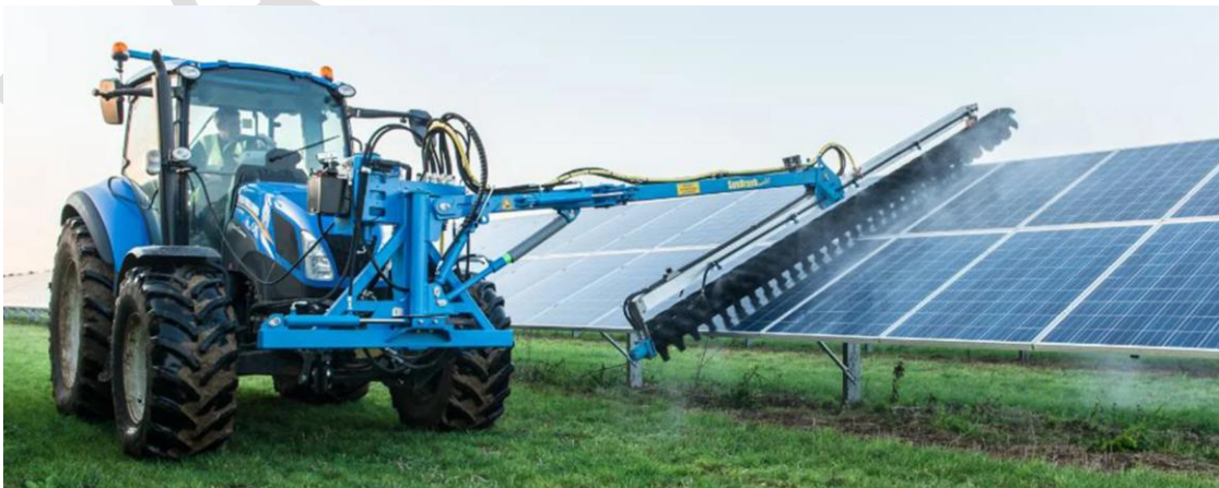
Photo 56: Cleaning of Solar Arrays
