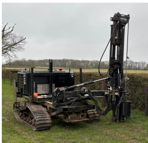
Photos 40 and 41: Example of Leg Piling and Panel Moving Equipment
